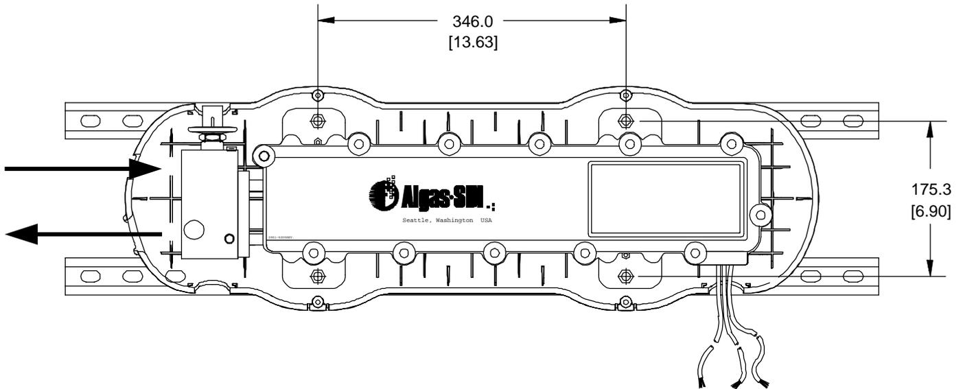
If mounted outdoors, the *Zimmer*<sup>TM</sup> must be mounted on a vertical and horizontal surface to maintain its enclosure rating. Use Algas-SDI Mounting Kit p/n **80885**, or equivalent components, when mounting the *Zimmer*<sup>TM</sup> to a concrete, masonry, or wood construction wall.
