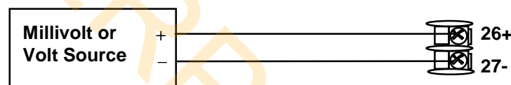
Figure 5-5 Wiring Connections for Radiamatic, Millivolts, Volts or Thermocouple Differential (Except 0 to 10 Volts)
