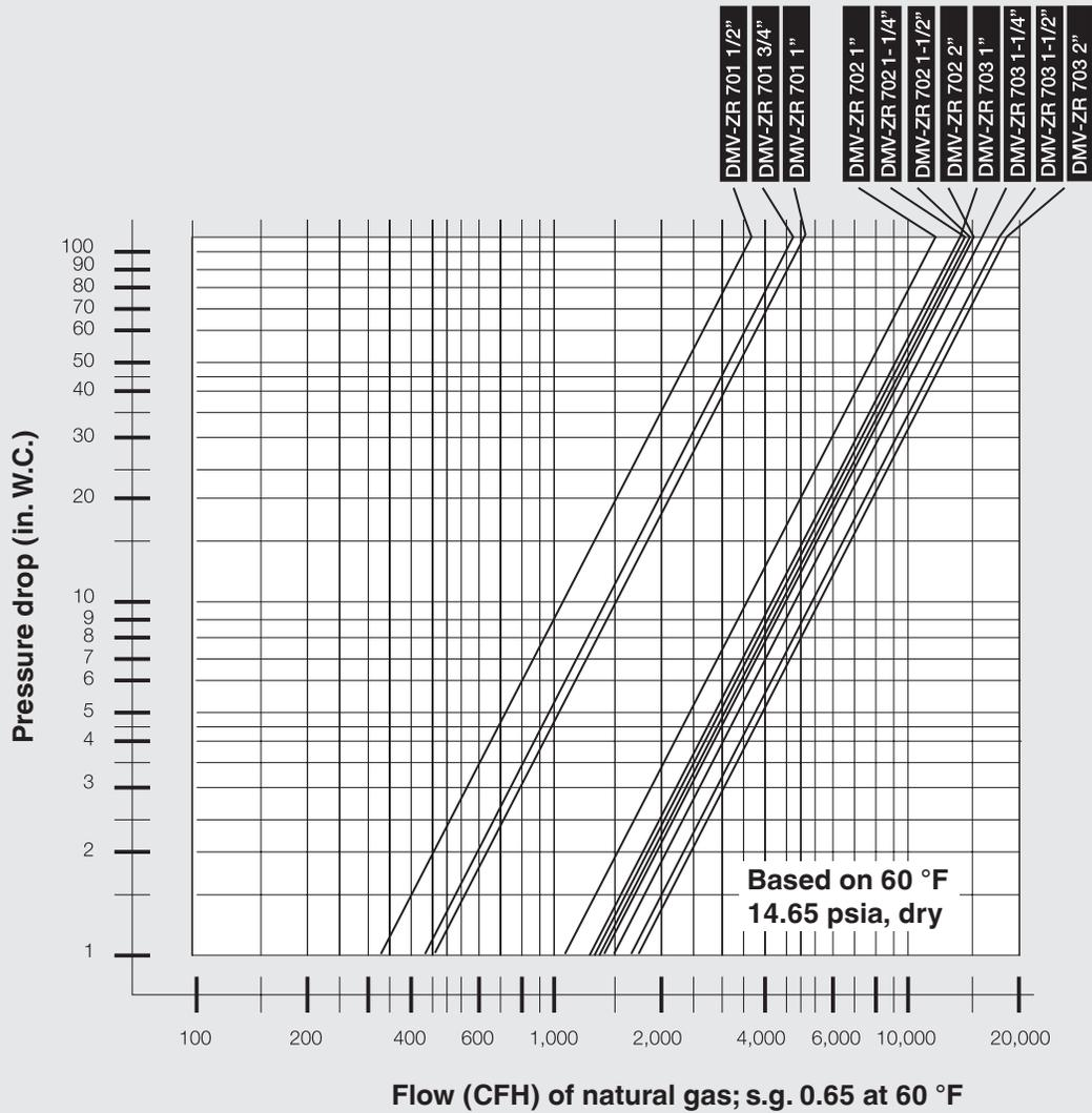
**⚠** Size valve for at least 2 in. W.C. of pressure drop or more if the inlet pressure in the application is 1/2 in. W.C. or less. Otherwise, the difference in flow rate between stage 1 and stage 2 will be noticeable.
