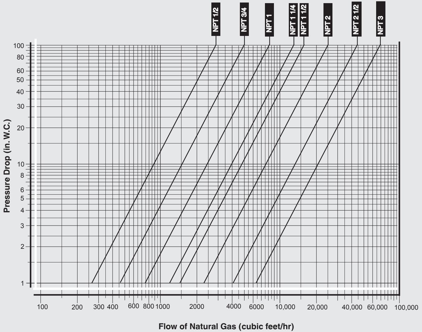
**Flow Curve Using Natural Gas for class II regulator.**
