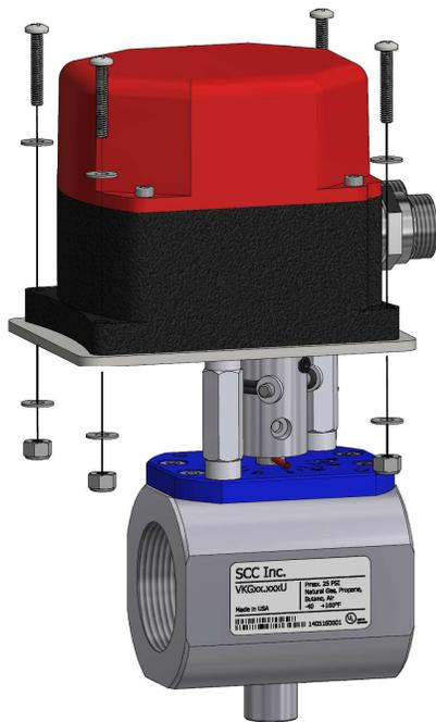
**Figure 5a: FX04 Actuator Installation**
