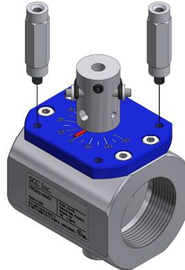
**Figure 3: Standoff Installation**
